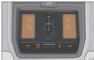
Fig. 98 Detail of roof lining: front lighting of the passenger compartment.
