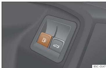
Fig. 212 Driver's door: tank flap release.
