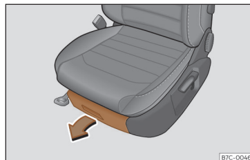
Fig. 139 Storage compartment under the front seats.
