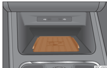
Fig. 151 In the centre console: pad for the mobile phone connection.
