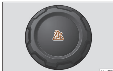
Fig. 224 Engine compartment: coolant expansion tank cap.
