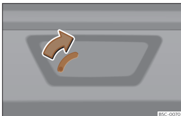
Fig. 91 Detail of the luggage compartment: manual release mechanism (Leon Sportstourer).
