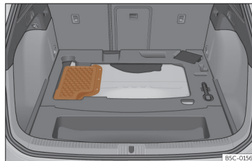
Fig. 227 Hybrid vehicles (PHEV): location of the battery in the luggage compartment
