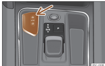
Fig. 75 Centre console: vehicle key socket.
