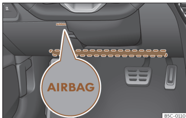
Fig. 21 On the driver side: location of the knee airbag
