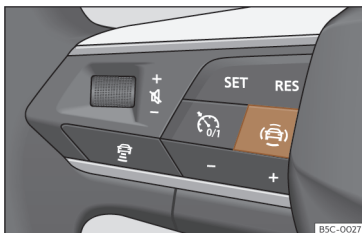
Fig. 66 Left side of the multifunction steering wheel: button for driver assistance systems (depending on versions).
