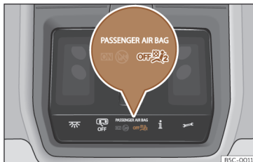
Fig. 20 On the roof console: control lamp for the deactivation of the front passenger front airbag.
