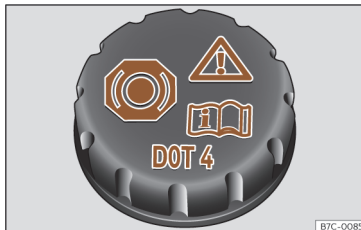
Fig. 225 Engine compartment: brake fluid reservoir cap.
