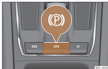
Fig. 187 In the lower part of the centre console: electronic parking brake button
