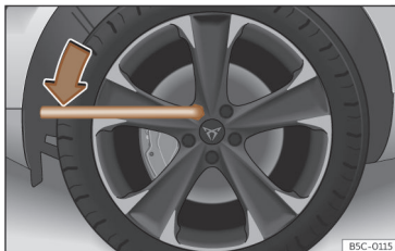
Fig. 233 Tyre change: slacken the wheel bolts.
