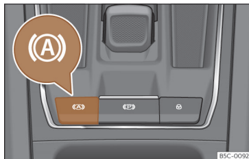
Fig. 146 In the lower part of the centre console: Auto Hold function button.
