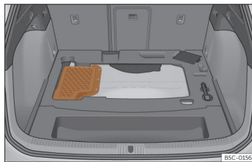
Fig. 224 Hybrid vehicles (PHEV): location of the battery in the luggage compartment
