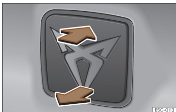
Fig. 75 Rear lid: opening from the outside.
