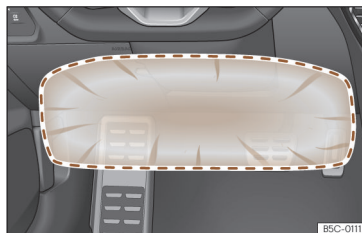
Fig. 37 On the driver side: action radius of airbag for knees.
