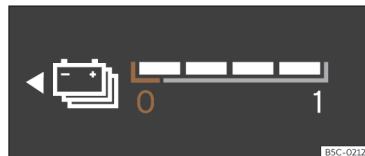
Fig. 5 Digital instrument cluster: battery level indicator.
