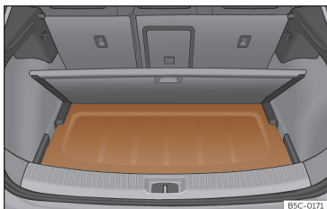
Fig. 174 In the boot: fitting the rear shelf.
