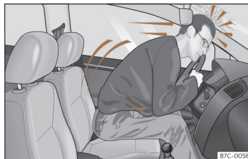
Fig. 21 A driver not wearing a seat belt may be thrown forward violently.
