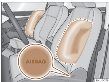
Fig. 33 Driver's seat and passenger seat side airbags.
