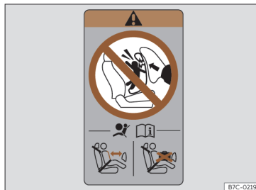
Fig. 40 Airbag sticker: on the rear frame of the passenger side door.
