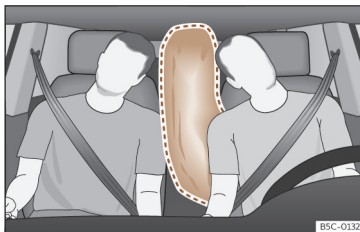
Fig. 32 Fully inflated central airbag (deployment zone).
