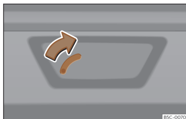
Fig. 80 Luggage compartment: manual release (Leon Sportstourer).
