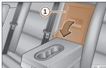
Fig. 190 On the rear seat backrest: opening the tailboard.
