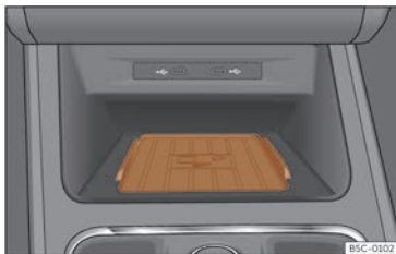
Fig. 170 Centre console: slot for mobile phone connection.
