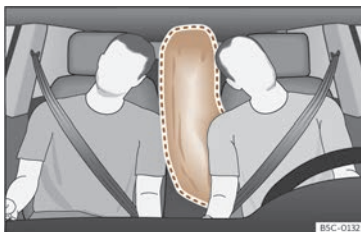
Fig. 32 Fully inflated central airbag (deployment zone).
