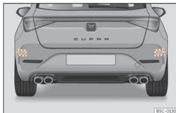
Fig. 124 Rear view of the vehicle: radar sensor areas.
