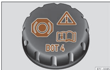
Fig. 218 Engine compartment: brake fluid reservoir cap.
