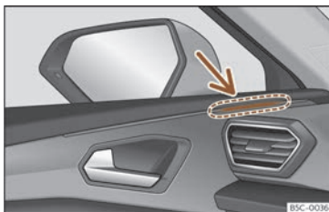
Fig. 141 Control lamp of the lane departure warning.
