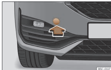
Fig. 206 Front bumper on right: remove the lid.
