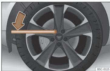
Fig. 234 Tyre change: slacken the wheel bolts.
