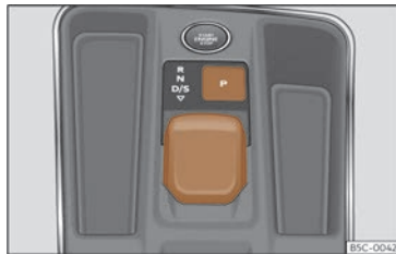
Fig. 115 On the centre console: selector lever.
