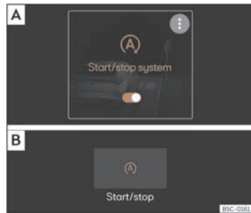
Fig. 113 On the infotainment system display: Start-Stop system on. A ) View in the main menu. B ) View with the Infotainment system off.
