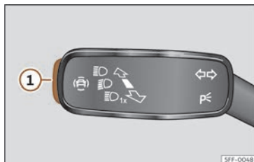
Fig. 119 On the turn light and main beam lever: key for driver assistance systems (depending on the version).
