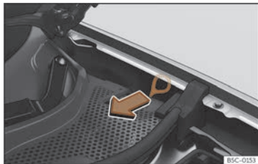
Fig. 59 Between the left wing panel and the engine bonnet hinge: Charging connector manual release mechanism puller.
