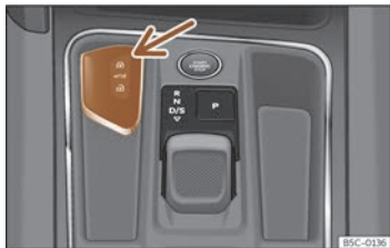
Fig. 64 Centre console: vehicle key housing.
