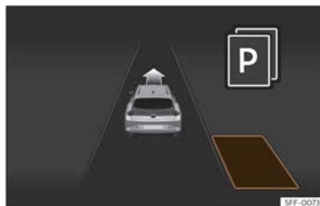
Fig. 149 On the instrument panel display: display of the assisted parking system with decreased visibility.
