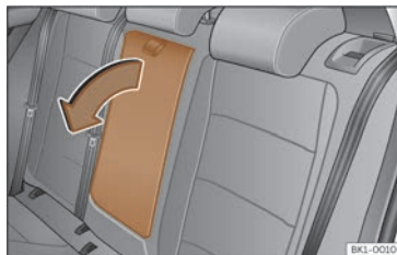
Fig. 97 Folding rear centre armrest (schematic view).
