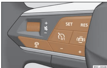
Fig. 130 On the multifunction steering wheel: buttons for operating the ACC.
