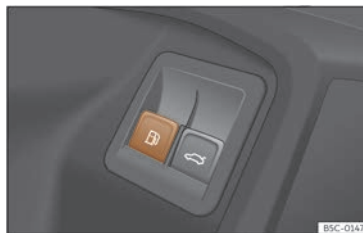
Fig. 200 Driver's door: tank cover release.
