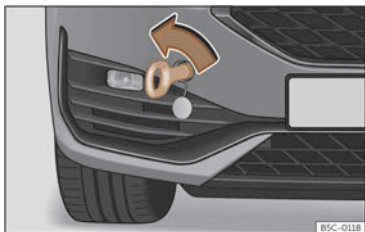
Fig. 207 Right side of the front bumper: towline anchorage screwed in.
