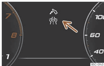
Fig. 10 Eco-efficient driving assistance indication (schematic representation).
