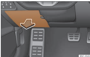
Fig. 210 On the dashboard on the driver side: lid of the fuse box.
