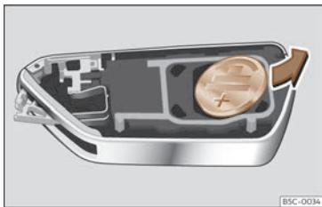
Fig. 67 Vehicle key: removing the battery.
