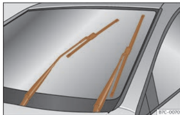
Fig. 203 Wipers in service position.
