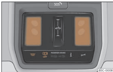
Fig. 101 Detail of headliner: front interior lighting.
