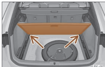
Fig. 180 Variable boot floor: tilted position.
