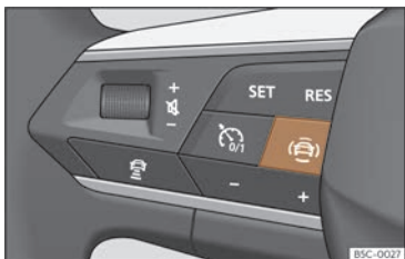
Fig. 120 Left side of the multifunction steering wheel: button for driver assistance systems (depending on the version).
