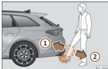
Fig. 78 Rear lid with sensor-controlled opening (Easy Open).
