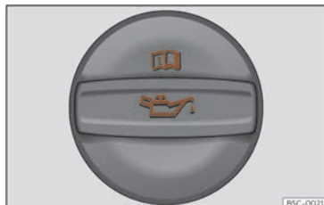
Fig. 223 Oil filler cap cover in the engine compartment.
