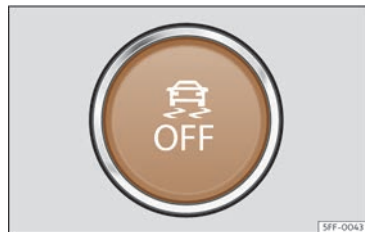
Fig. 118 On the lower part of the centre console: ESC on/off button
