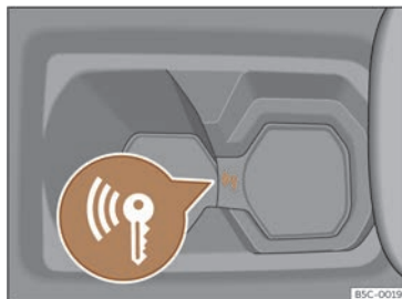
Fig. 112 On the centre console: emergency start.
