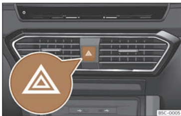
Fig. 49 Dashboard: switch for hazard warning lights.
