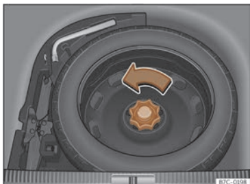
Fig. 230 In the luggage compartment: raised load floor.
