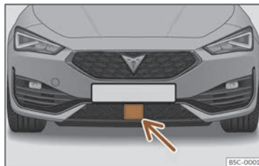
Fig. 121 On the front bumper: radar sensor.
