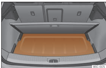
Fig. 174 In the boot: fitting the rear shelf.
