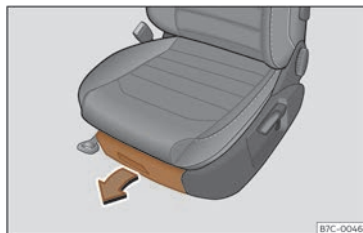
Fig. 160 Storage compartment under the front seats.
