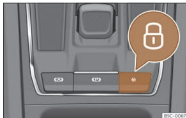
Fig. 71 On the centre console: central locking switch
