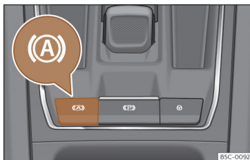
Fig. 188 In the lower part of the centre console: Auto Hold function button.
