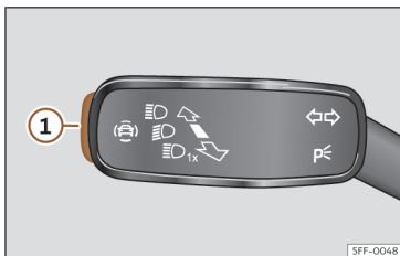
Fig. 65 On the turn signal and main beam lever: button for driver assistance systems (depending on versions).
