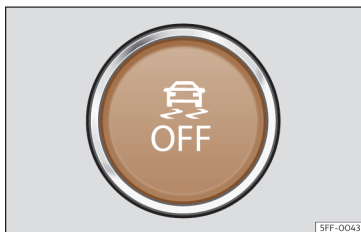
Fig. 189 In the lower part of the centre console: button to switch the ESC off/on
