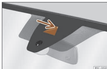
Fig. 124 On the windscreen: field of vision of the Lane Assist system camera.
