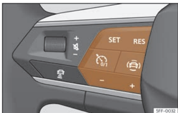
Fig. 129 On the multifunction steering wheel: buttons to control the speed limiter.
