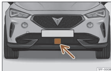
Fig. 122 On the front bumper: radar sensor.
