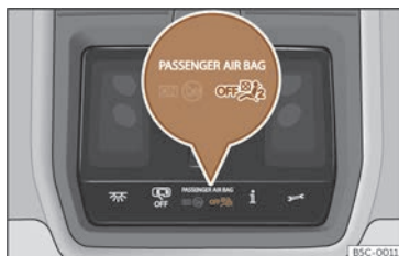
Fig. 30 On the roof console: passenger airbag deactivation control lamp.
