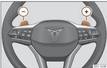
Fig. 117 Steering wheel: automatic gearbox levers
