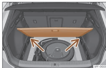
Fig. 178 Variable boot floor: tilted position.
