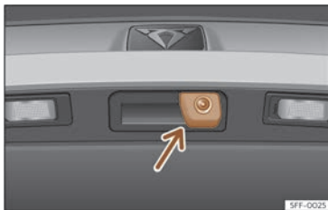
Fig. 127 On the rear lid handle: location of the rear assist camera.
