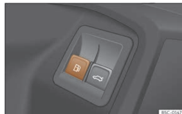
Fig. 192 Driver's door: tank cover release.
