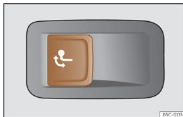
Fig. 187 Left side of the luggage compartment: button to unlock the tow hitch.
