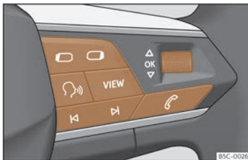
Fig. 11 Right side of multifunction steering wheel: buttons to the menus and informative indications on the instrument panel (depending on the version).
