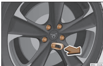
Fig. 224 Wheel: wheel bolts with caps.
