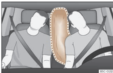
Fig. 32 Fully inflated central airbag (deployment zone).
