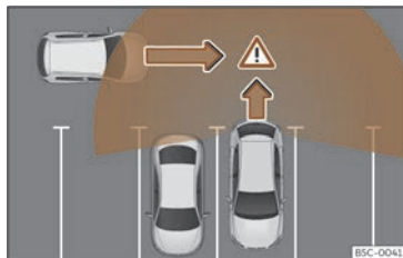
Fig. 157 Diagram of the parking assistant: detected area around the vehicle that is driving off.
