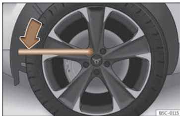
Fig. 226 Tyre change: slacken the wheel bolts.
