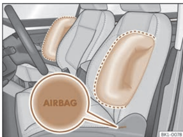
Fig. 33 Driver's seat and passenger seat side airbags.
