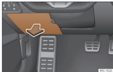
Fig. 203 On the dashboard on the driver side: lid of the fuse box.
