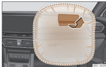
Fig. 28 Front passenger airbag located in dash panel.
