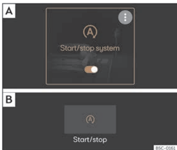
Fig. 114 On the infotainment system display: Start-Stop system on. A View in the main menu. B View with the Infotainment system off.
