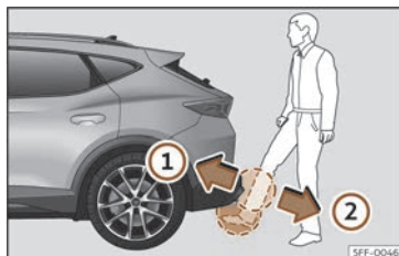
Fig. 78 Rear lid with sensor-controlled opening (Easy Open).
