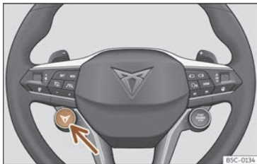
Fig. 118 Multifunction steering wheel: button to change the driving profile.
