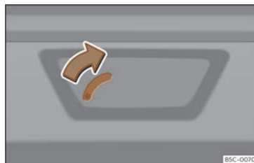
Fig. 80 Luggage compartment: manual release.
