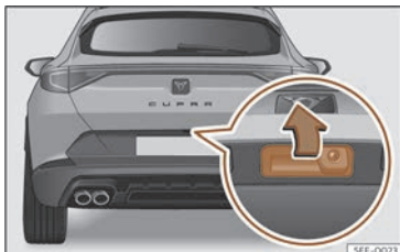
Fig. 75 Rear lid: opening from the outside.
