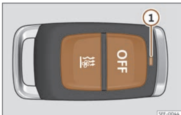
Fig. 111 Independent heating: radiofrequency remote control key
