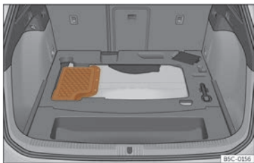
Fig. 217 Hybrid vehicles (PHEV): location of the battery in the luggage compartment
