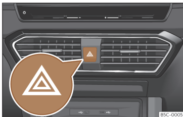
Fig. 94 Dash panel: hazard warning lights switch
