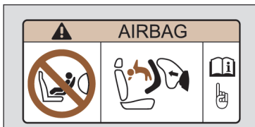
Fig. 25 Airbag sticker: on the passenger's sun visor
