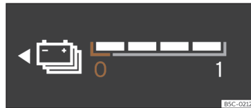
Fig. 59 Digital instrument panel: battery level indicator.
