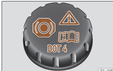
Fig. 219 Engine compartment: brake fluid reservoir cap.
