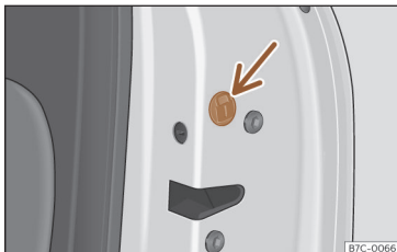
Fig. 81 Locking the door manually.
