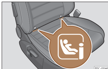
Fig. 28 Front passenger seat: ISOFIX/i-Size securing rings.
