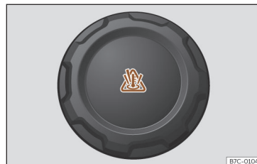
Fig. 218 Engine compartment: coolant expansion tank cap.
