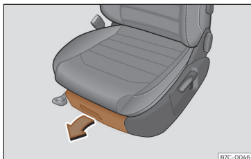
Fig. 127 Storage compartment under the front seats.
