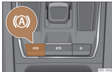
Fig. 178 In the lower part of the centre console: Auto Hold function button.
