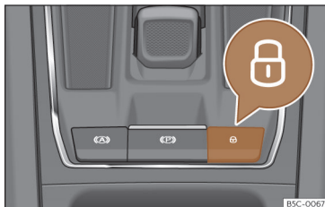
Fig. 77 In the centre console: central locking switch
