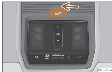
Fig. 32 On the roof console: voice service controls
