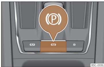
Fig. 177 In the lower part of the centre console: electronic parking brake button
