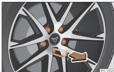
Fig. 36 Wheel: wheel nuts with caps.
