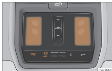
Fig. 95 Detail of roof lining: front lighting of the passenger compartment.
