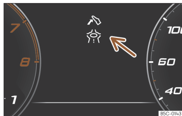
Fig. 56 Eco-efficient driving assistance indication (schematic representation).
