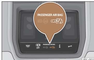
Fig. 16 On the roof console: control lamp for the deactivation of the front passenger front airbag.
