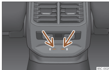
Fig. 140 Rear part of the centre console: USB connectors with power outlet function.
