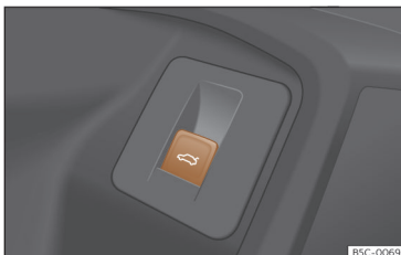
Fig. 84 On the driver's door: button to open and close the rear lid.
