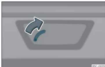
Fig. 85 Detail of the luggage compartment: emergency unlocking
