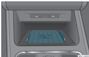
Fig. 135 In the centre console: pad for the mobile phone connection.
