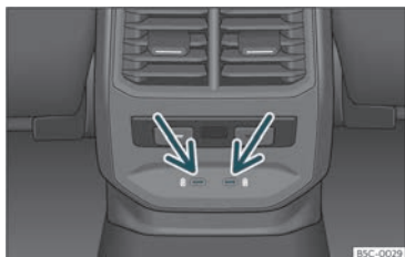
Fig. 137 Rear part of the centre console: USB connectors with power outlet function.
