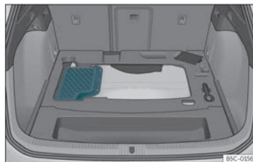
Fig. 211 Location of the battery in the luggage compartment
