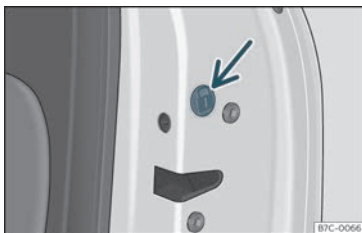
Fig. 79 Locking the door manually.
