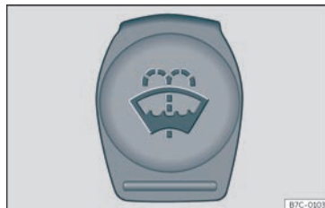
Fig. 209 In the engine compartment: window washer tank cap.
