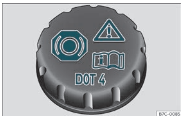
Fig. 208 Engine compartment: brake fluid reservoir cap.
