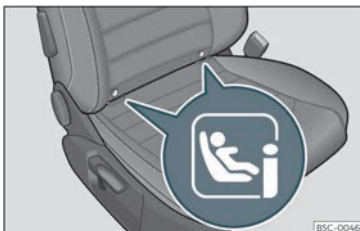
Fig. 28 Front passenger seat: ISOFIX/i-Size securing rings.
