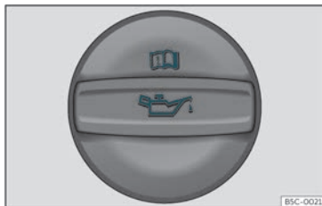
Fig. 204 In the engine compartment: Engine oil filler cap.
