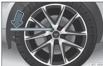
Fig. 37 Wheel change: loosen the wheel nuts.
