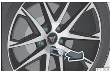
Fig. 35 Wheel: wheel nuts with caps.
