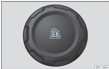
Fig. 207 Engine compartment: coolant expansion tank cap.
