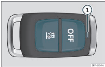
Fig. 129 Auxiliary heating: radio-operated remote control.
