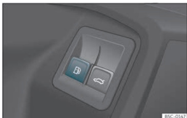
Fig. 196 Driver's door: tank flap release.
