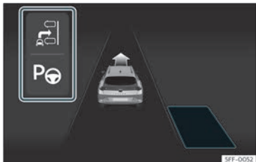
Fig. 175 On the instrument panel display: view of the parking assist system with reduced view.
