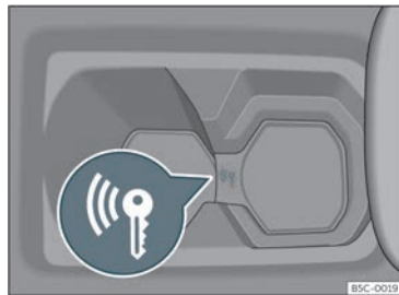
Fig. 139 In the centre console: emergency start.
