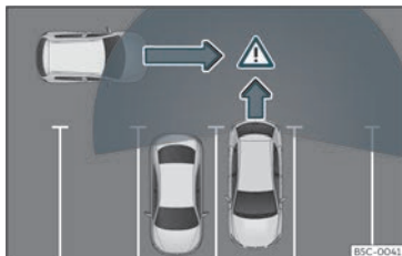
Fig. 169 Schematic representation of the rear cross traffic alert assistant: zone monitored around the vehicle while leaving a parking space.
