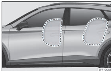
Fig. 22 Illustration of completely inflated side airbags on the left side of the vehicle.
