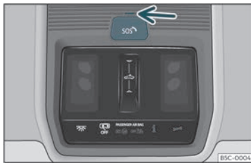
Fig. 32 On the roof console: voice service controls
