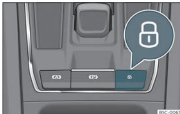
Fig. 75 In the centre console: central locking switch
