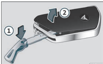
Fig. 72 Vehicle key: opening the battery compartment cover.
