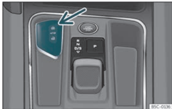
Fig. 70 Centre console: vehicle key socket.
