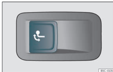
Fig. 185 On the left side of the luggage compartment: button for unlocking the tow hook.
