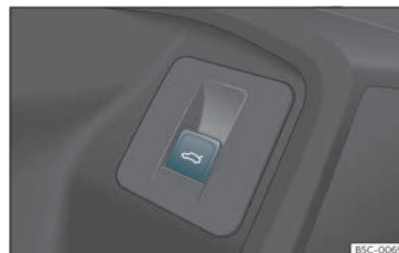
Fig. 83 On the driver's door: button to open and close the rear lid.
