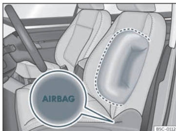
Fig. 21 Side airbag in driver's seat.
