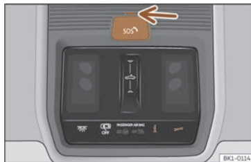
Fig. 61 On the roof console: controls for voice services.
