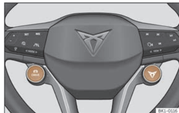
Fig. 117 Multifunction steering wheel: DRIVE and CUPRA buttons for selecting and changing the driving profile.
