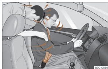
Fig. 36 Any rear seat occupants not wearing a seat belt may be thrown forward violently, hitting the driver who is wearing the seat belt.
