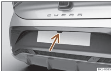
Fig. 123 On the rear bumper: location of the rear assist camera.
