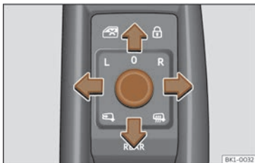
Fig. 110 Detail of the driver door: control for the exterior mirror.
