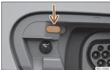
Fig. 70 Behind the battery charging socket cover: charging process indicator.
