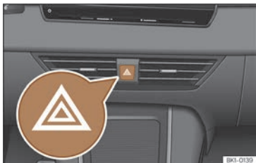
Fig. 60 Dashboard: switch for hazard warning lights.
