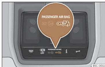
Fig. 44 On the roof console: passenger airbag deactivation control lamp.
