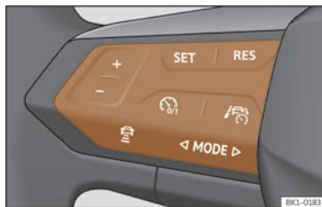
Fig. 124 On the multifunction steering wheel: buttons to control the speed limiter.
