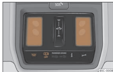
Fig. 105 Detail of headliner: front interior lighting.
