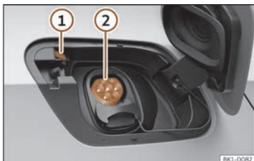
Fig. 68 Behind the battery charging cover on the rear right-hand side: Charging socket
