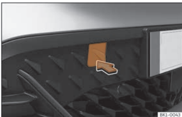
Fig. 183 Front bumper on right: remove the lid.
