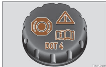
Fig. 193 Front compartment: brake fluid reservoir cap.
