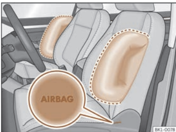
Fig. 47 Driver's seat and passenger seat side airbags.
