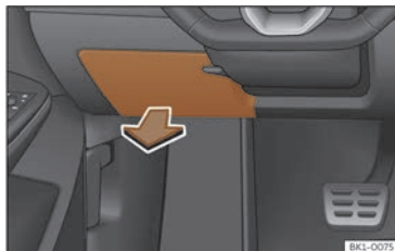
Fig. 185 On the dashboard on the driver side: lid of the fuse box.
