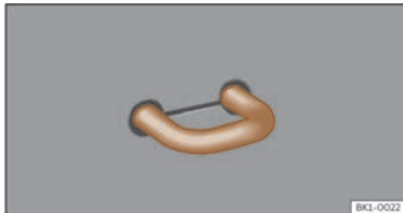
Fig. 173 In the luggage compartment: fastening rings.
