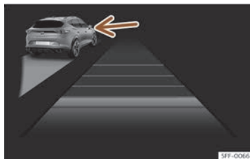
Fig. 127 On the instrument panel display: ACC active, vehicle detected on the left.
