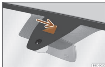
Fig. 120 On the windscreen: field of vision of the Lane Assist system camera.
