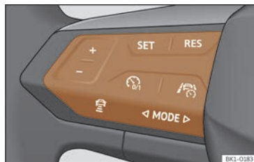
Fig. 126 On the multifunction steering wheel: buttons for operating the ACC.
