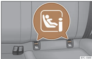
Fig. 52 Rear seat: location of the ISOFIX or i-Size securing rings.
