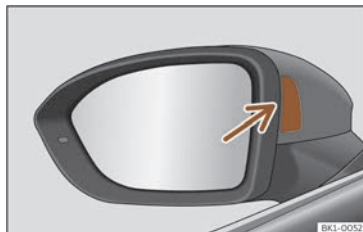
Fig. 156 On the mirror: warning lamp.
