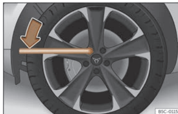
Fig. 200 Tyre change: slacken the wheel bolts.
