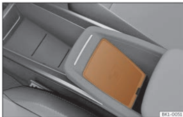
Fig. 167 Centre console: slot for mobile phone connection.
