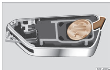
Fig. 81 Vehicle key: removing the battery.
