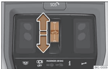
Fig. 112 On the interior roof lining: function button to operate the sun blind.
