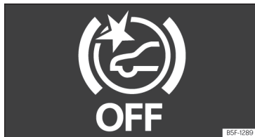
Fig. 132 On the screen of the instrument panel Front Assist switched off message.
