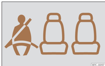
Fig. 34 Instrument cluster: indication of the status of the rear seat seat belts.
