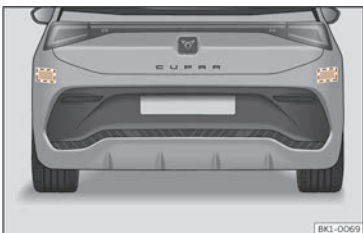
Fig. 121 Rear view of the vehicle: radar sensor areas.
