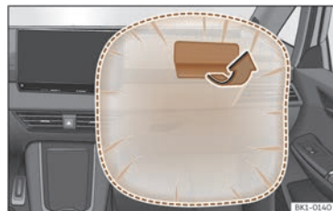
Fig. 42 Front passenger airbag located in dash panel.
