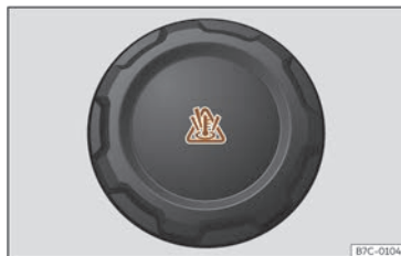
Fig. 192 Front compartment: coolant expansion tank cap.
