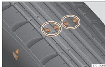
Fig. 196 Tyre profile: tread wear indicators.
