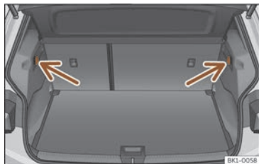
Fig. 174 In the boot: retaining hooks.
