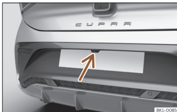
Fig. 126 On the rear bumper: location of the rear assist camera.
