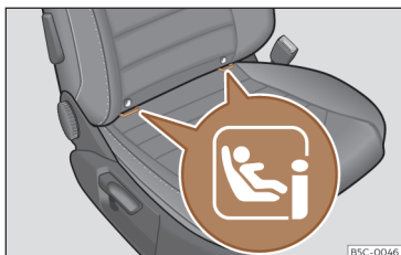
Fig. 59 Front passenger seat: i-Size fastening rings.
