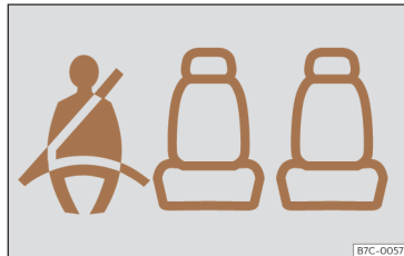
Fig. 38 Instrument cluster: indication of the status of the rear seat seat belts.
