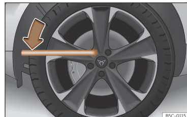
Fig. 200 Tyre change: slacken the wheel bolts.
