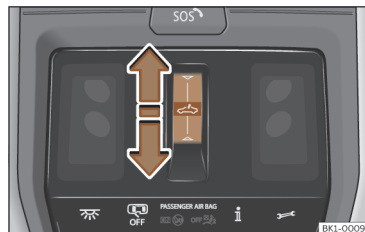
Fig. 115 On the interior roof lining: function button to operate the sun blind.
