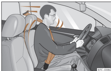
Fig. 39 Drivers with properly worn seat belts will not be thrown forward in the event of sudden braking.
