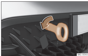
Fig. 184 Right side of the front bumper: towline anchorage screwed in.
