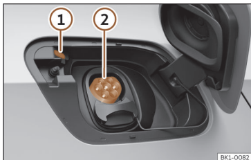
Fig. 72 Behind the battery charging cover on the rear right-hand side: Charging socket.
