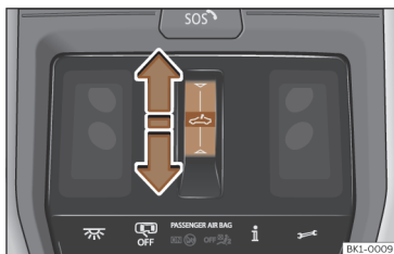
Fig. 90 On the interior roof lining: function button for operating the sun blind.
