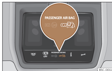
Fig. 26 On the roof console: control lamp for the deactivation of the front passenger front airbag.
