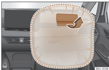
Fig. 24 Front passenger airbag located in dash panel.
