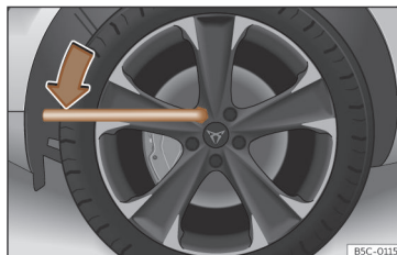
Fig. 167 Wheel change: loosen the wheel nuts.
