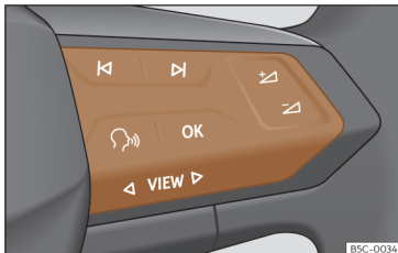
Fig. 71 Controls on the steering wheel.
