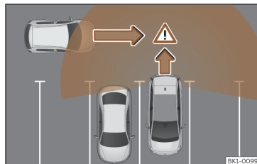
Fig. 115 Schematic representation of the rear cross traffic alert assistant: zone monitored around the vehicle while leaving a parking space.
