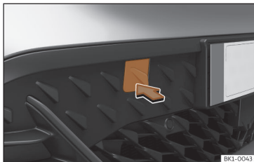
Fig. 149 On the right side of the front bumper: remove the cover.
