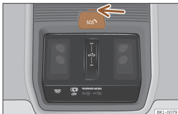
Fig. 41 On the roof console: voice service controls
