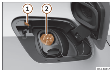
Fig. 48 Behind the battery charging cover on the rear right-hand side: Charging socket
