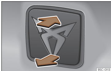
Fig. 67 Rear lid: opening from outside.
