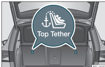
Fig. 34 Position of the Top Tether rings on the back of the rear seat.
