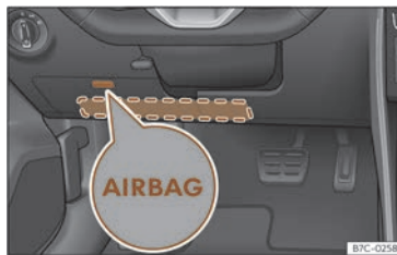
Fig. 30 On the driver side: location of airbag for knees.
