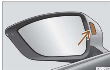
Fig. 120 Control lamp of the lane departure warning.
