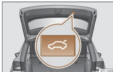
Fig. 55 Rear lid: button to close rear lid.
