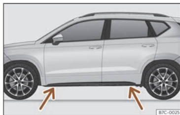
Fig. 210 Jack position points.
