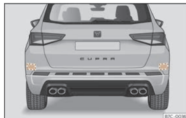
Fig. 104 Rear view of the vehicle: radar sensor areas.
