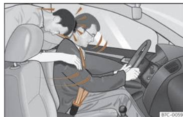
Fig. 18 Any rear seat occupants not wearing a seat belt may be thrown forward violently, hitting the driver who is wearing the seat belt.
