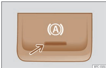
Fig. 125 In the lower part of the centre console: Auto Hold function button.
