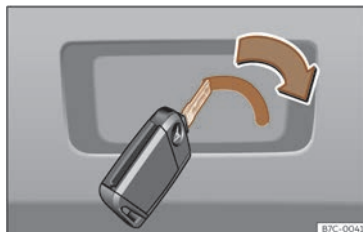
Fig. 59 Luggage compartment: manual release.
