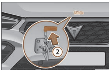
Fig. 192 Lever under the bonnet.
