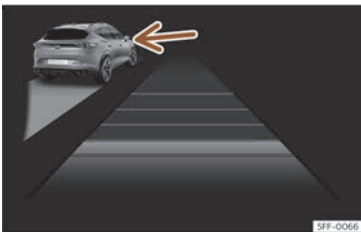
Fig. 111 On the instrument panel display: ACC active, vehicle detected on the left.
