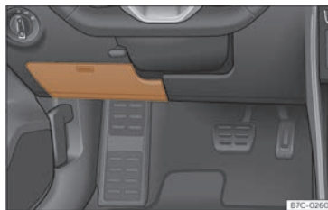
Fig. 187 On the dashboard on the driver side: lid of the fuse box.
