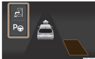
Fig. 132 On the instrument panel display: display of the assisted parking system with decreased visibility.
