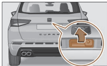
Fig. 54 Rear lid: opening from the outside.
