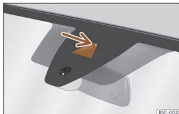
Fig. 103 On the windscreen: field of vision of the Lane Assist system camera.
