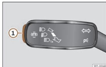
Fig. 99 On the turn light and main beam lever: key for driver assistance systems (depending on the version).
