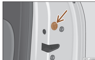
Fig. 75 Locking the door manually.
