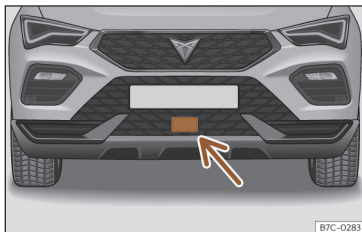
Fig. 145 On the front bumper: radar sensors.
