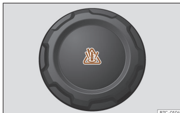
Fig. 203 Engine compartment: coolant expansion tank cap.
