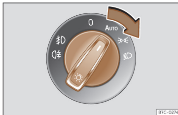
Fig. 87 Dash panel: lights control.
