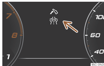
Fig. 53 Eco-efficient driving assistance indication (schematic representation).
