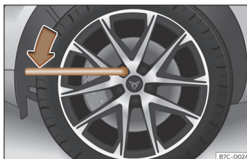
Fig. 34 Wheel change: loosen the wheel nuts.
