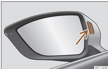
Fig. 165 Control lamp of the lane departure warning.
