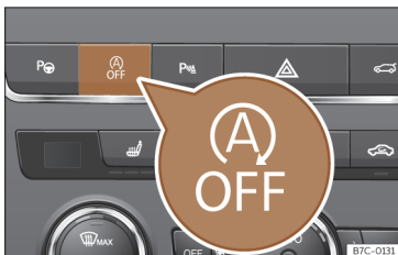
Fig. 138 Centre console: Start-stop system button.
