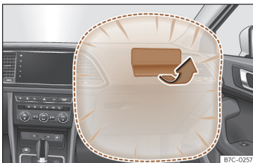
Fig. 14 Front passenger airbag located in dash panel.
