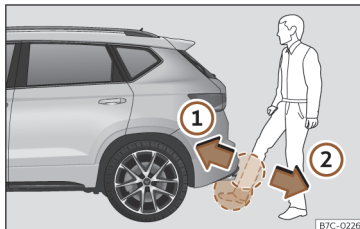
Fig. 80 Rear lid with sensor-controlled opening (Easy Open).
