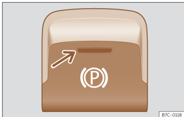
Fig. 170 In the lower part of the centre console: electronic parking brake button
