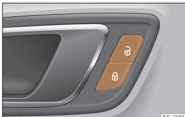
Fig. 70 Driver's door: central locking switch.
