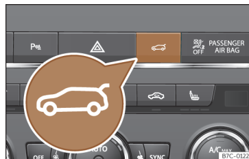
Fig. 79 Centre console: button to open and close the rear lid.
