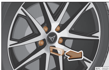
Fig. 32 Wheel: wheel nuts with caps.
