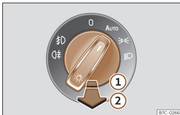
Fig. 88 Dash panel: lights control.
