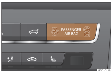
Fig. 16 Dash panel: control lamp for the deactivation of the front passenger front airbag.
