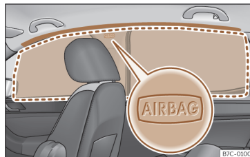
Fig. 21 Location of head-protection airbags.
