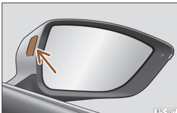
Fig. 166 Control lamp of the lane departure warning.
