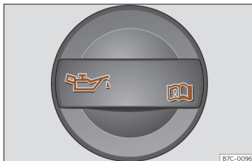
Fig. 201 In the engine compartment: Engine oil filler cap.
