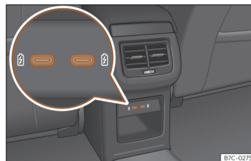
Fig. 135 Rear part of the centre console: USB connectors with power outlet function.
