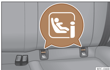
Fig. 25 Rear seat: ISOFIX/i-Size securing rings.
