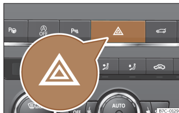
Fig. 90 Dash panel: hazard warning lights switch
