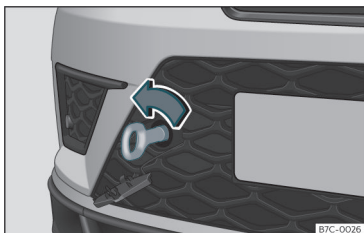
Fig. 40 On the right side of the front bumper: towline anchorage in position.
