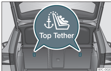
Fig. 33 Position of the Top Tether rings on the back of the rear seat.
