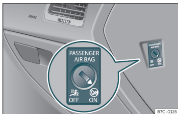
Fig. 22 Front passenger front airbag switch.
