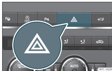
Fig. 121 Dashboard: switch for hazard warning lights.
