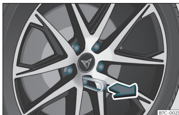
Fig. 59 Wheel: wheel bolts with caps.
