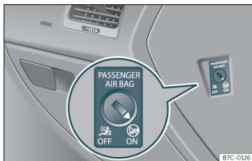
Fig. 81 Switch for activating and deactivating the front passenger airbag.
