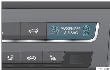
Fig. 23 Dashboard: control lamp for deactivated front passenger airbag in centre console.
