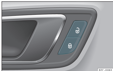
Fig. 2 Driver door: central locking switch.
