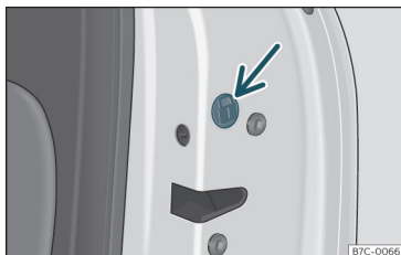
Fig. 4 Locking the door manually.
