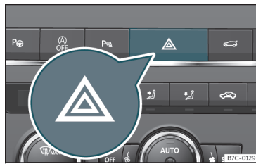
Fig. 39 Dashboard: switch for hazard warning lights.
