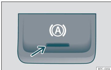
Fig. 201 In the lower part of the centre console: Auto Hold function button.
