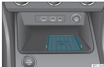
Fig. 193 Centre console: slot for mobile phone connection.
