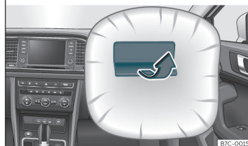
Fig. 21 Front passenger airbag located in dash panel.
