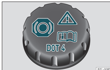
Fig. 52 Engine compartment: brake fluid reservoir cap.
