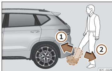
Fig. 80 Rear lid with sensor-controlled opening (Easy Open).
