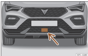
Fig. 143 On the front bumper: radar sensors.
