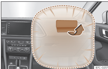
Fig. 14 Front passenger airbag located in dash panel.
