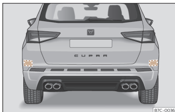
Fig. 146 Rear view of the vehicle: radar sensor zones.
