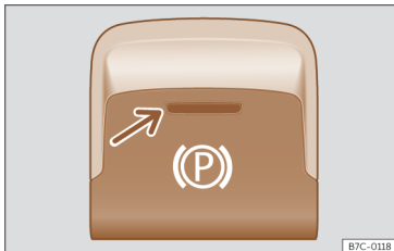
Fig. 168 In the lower part of the centre console: electronic parking brake button
