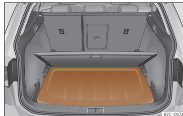
Fig. 108 In the luggage compartment: fitting the rear shelf.
